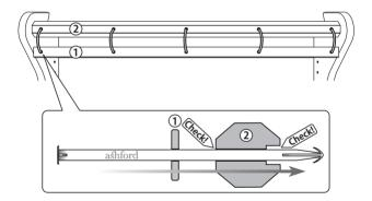
Connect the warp sticks to the roller with the warp stick ties. First push the arrow head through the warp stick. Then push the arrow head into the small hole in the roller and out the large hole as illustrated.
