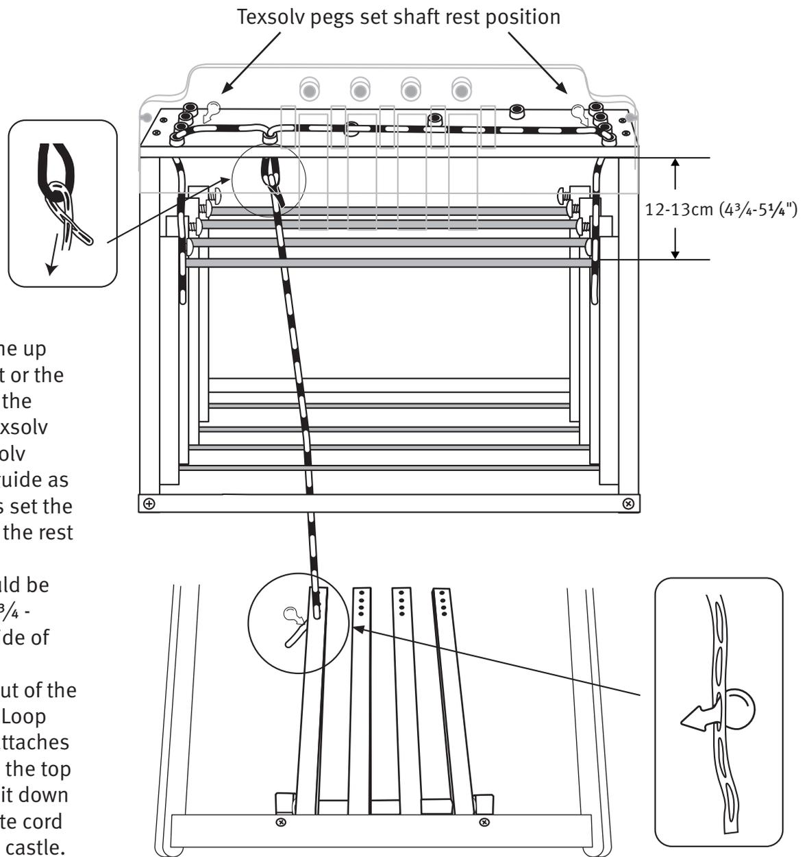
Move the levers into the up position on the 4 shaft or the 4 right hand levers on the 8 shaft loom. Insert Texsolv pegs through the Texsolv cord beside the cord guide as illustrated. These pegs set the height of the shafts in the rest position.
