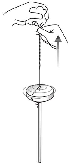
**4** Slowly slide your fingers back up the drafted fibres allowing the twist to follow. Once twisted, the yarn will support the weight of the spindle.
