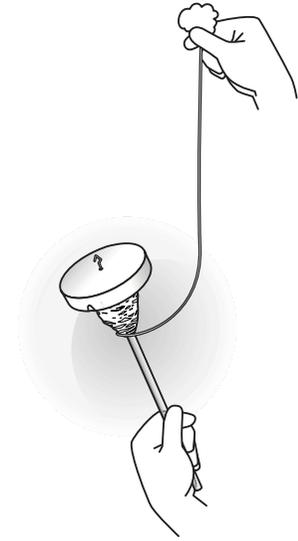
**6** Wind the yarn around the shaft to form a cone & then repeat the process. Slide the cone off the shaft and use either as a single or ply 2 together with the spindle spinning anti-clockwise.
