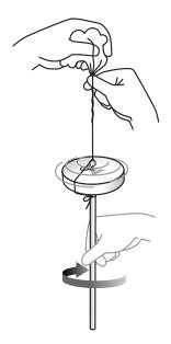
Spin the spindle clockwise and allow the leader to join onto your prepared fibres.
