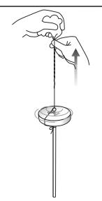
Slowly slide your fingers back up the drafted fibres allowing the twist to follow. Once twisted, the yarn will support the weight of the spindle.
