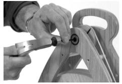
**5.** Lift the back frame away from the flyer shaft and crank.
