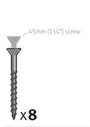
120cm (48") wide loom: Use the 45mm (1<sup>3</sup>/<sub>4</sub>") screws.
