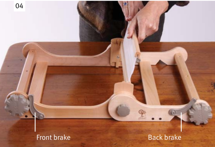
Place the reed into the rest position. Make sure the front and back brakes are on. When we say put the brake on, we mean the pawl should be clicked into the ratchet on the handle.
