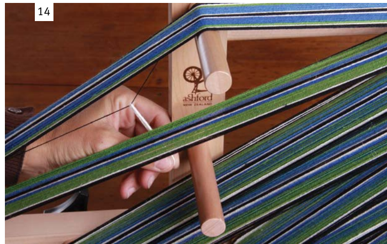
14 Slip the loops onto the leash peg. NOTE: leashes are only on top threads (Round 1 threads).
