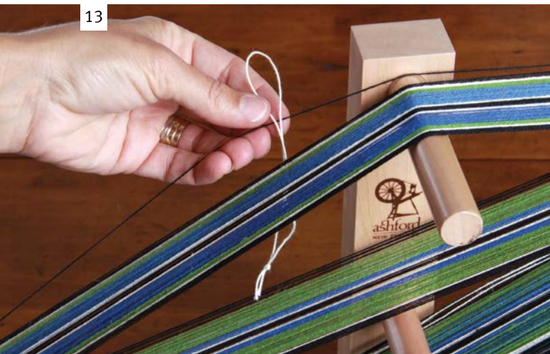
13 Adding the leashes. Take a leash up and over the first thread of the warp (Round 1 thread).
