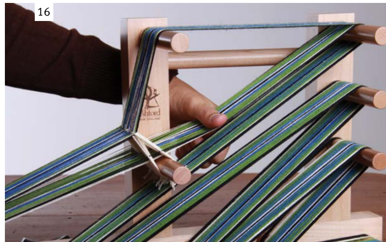
16 Shed 1: Push the threads down to create a space (shed) in front of the leashes.
