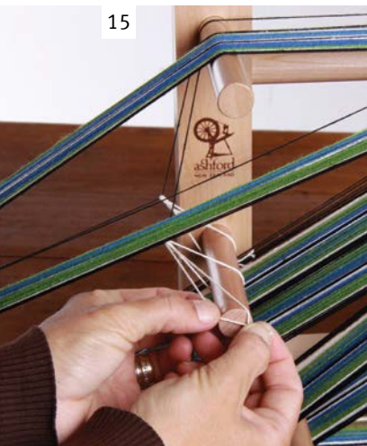
15 Continue across the warp adding leashes to all Round 1 threads. Keeping your threads in order , you should have Round 1 with a leash, then the Round 2 thread, then the next Round 1 with a leash and so on. NOTE: Use the top rear peg to sort through the threads as you add the leashes.
