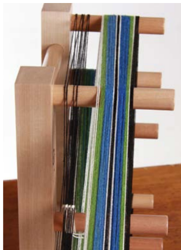
15 Continue across the warp adding leashes to all Round 1 threads. Keeping your threads in order , you should have Round 1 with a leash, then the Round 2 thread, then the next Round 1 with a leash and so on. NOTE: Use the top rear peg to sort through the threads as you add the leashes.
