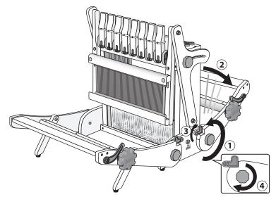
**Step 4:** Loosen knobs securing the beater supports, slide the beater completely forward and tighten the knobs. *NOTE:* To avoid potential damage to the top beater rail we have packed it separately. Please attach it to the beater arms with 2 x bolts, washers and wing nuts. Make sure the wing nuts are parallel to the beater rails to ensure the loom folds.
