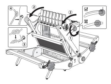
**Step 6:** Push the levers down and check the gap between the shafts and the castle top is approx.  $1 \text{ cm} (\frac{1}{2} \text{ ins})$  on both sides. Adjust the height as necessary by moving the Texsolv cord in the lever or on the screw head in the shaft end.
