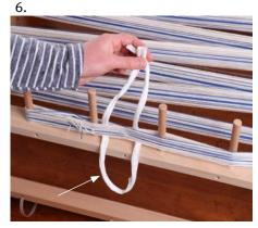
When all the yarn has been wound on, add choke ties to the warp to prevent tangling. Add a long loose tie through each side of the threading cross.
