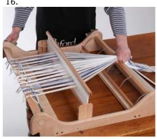
Untie the warp from the front roller. Now it's time to wind the yarn onto the back roller, keep the warp under tension. A friend can help by holding the end of the chain out under tension at the front of the loom.
