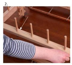
Tie the warp yarn to the start peg with a loop. Wind around the pegs for the required warp length and return following the same path back to the beginning.
