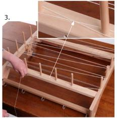
When returning back to the start you will be creating a threading cross between the second to last peg spacing. Create this cross by passing the thread up or down in the opposite direction to the previous thread. The threading cross keeps the yarn in the correct order for threading.
