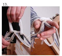
Pick up the threading cross and insert your fingers on either side of the cross. Then remove the choke tie by the threading cross.
