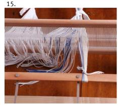
Once all the warp yarns are threaded through each slot and eye, tie them to the back warp stick in small bunches.
