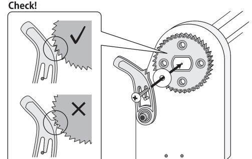
Locate the 4 pins on the handle into the 4 holes in the cog. Then give the handle a sharp hit with your fist so it snaps down tight onto the cog. When you are ready to advance the warp, release the warp tension by turning the handle slightly and then lifting the pawl out of the teeth.
