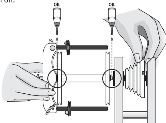
2. Thread the flyer spindle into the top shaft. Hold the flyer whorl with one hand and rotate the flyer clockwise with the other. Take care not to force or overtighten the flyer.
