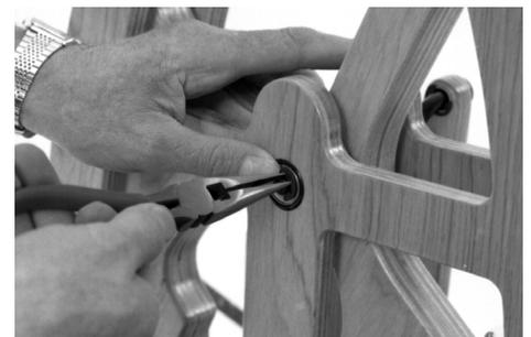
9. Replace the screws holding the back frame to the base and dowel spacers.
