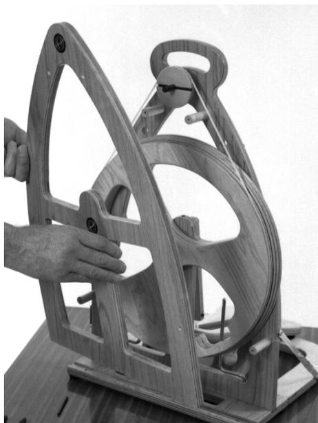
6. Carefully remove the E-Clip from the front of the flyer shaft and slide the shaft out. Carefully remove the E-Clip from in front of the pulley and slide the pulley off the shaft. Tap the tension pin out of the original flyer shaft and tap it into the new flyer shaft. Slide the pulley onto the new flyer shaft until the groove engages the tension pin. Then secure with an E-Clip. Fit the new shaft into the frame and secure with an E-Clip.
