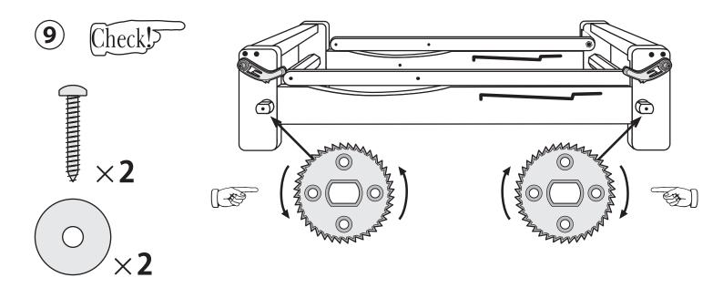
Place the cogs onto the ends of the rollers. Check the teeth engage the pawl. THEN secure with washers with small holes and 25mm (1") screws.
