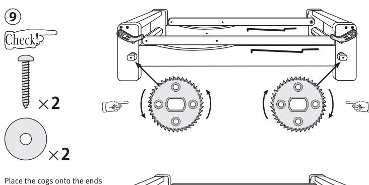
Place the cogs onto the ends of the rollers. Check the teeth engage the pawl. THEN secure with washers with small holes and 25mm (1") screws.
