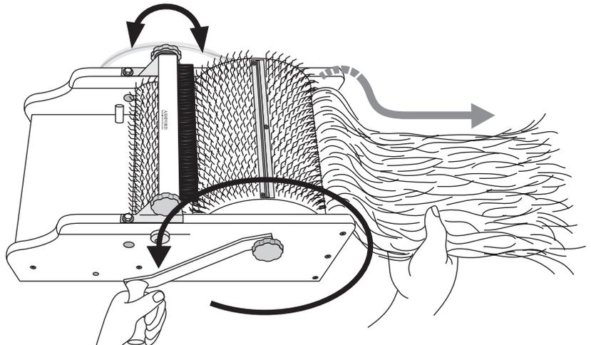
Remove the batt, clean the drums as necessary, reposition the brush into the carder teeth and tighten the 2 knobs. Experiment with the position of the packer brush to best suit the fibre you are carding.
