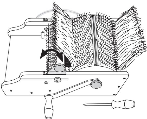
When the large drum is full or fibre starts collecting on the small drum, loosen the 2 knobs and twist the packer brush up out of the teeth.
