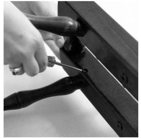
7. Locate one end of the double treadle rail into the hole in the leg in the base. Place the other leg onto the other end. Push the leg back into the base. Check the treadle rail moves freely. Hammer the leg in and secure with the screw.
